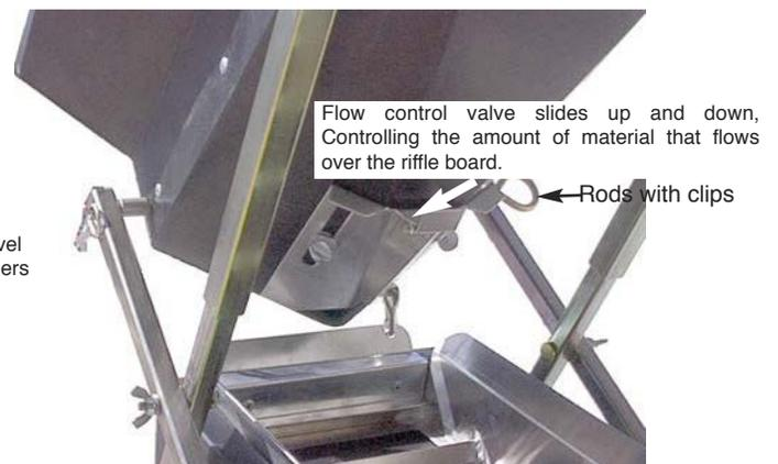
Secure the air duct hose to the bottom of the recovery box assembly and engine blower assembly with hose clamps. Check oil and fuel level and then start engine. Start shoveling material into the hopper and adjust the flow control valve so that a smooth even flow of material passes over the riffles. Adjust concentrator tray angle for a slow constant flow of material. See written instructions for more detail on general operation.
