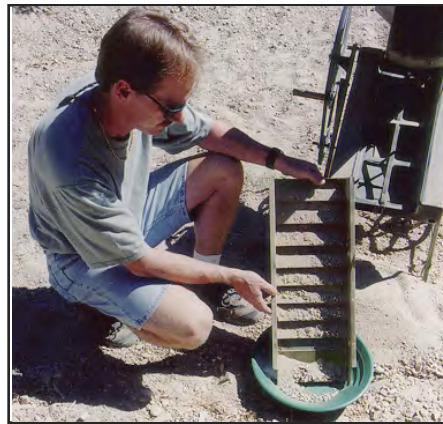
Cleaning the recovery tray into a gold pan to check the occurrence of gold in the concentrates.
