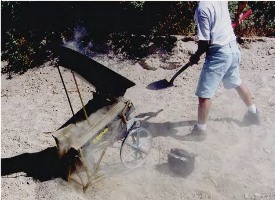
Keene Engineering Model DW212V Battery Operated Dry Washer
