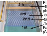
Placement of screens and matting in sluice box
