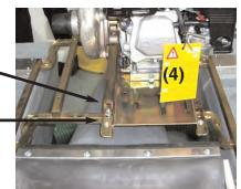
**3.** Mount engine onto frame as per diagram above (fig 4). Attach base plate to frame using four engine bolts. Sometimes only three bolts are necessary when adapting a compressor.
