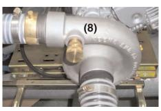
Attach suction tip to suction hose with hose clamp (fig 6). (We recommend to cover hose clamp with a type of duct or friction tape to prevent potential injury from sharp extruding objects)
