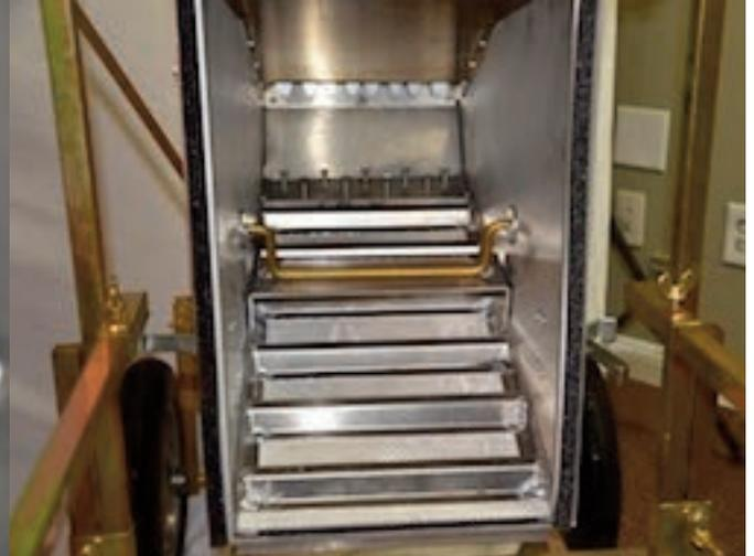
This picture shows the riffle board in place and the riffle board locked down with the locking cam. The riffle faces towards from the opening for dry washing It is important to place the riffle cartridge in correctly so that the Lexan openings inside the riffle cartridge lines up with the aluminum support base openings. If it is not lined up this can cause the dead air spaces to be off and can effect the fine gold recovery.
