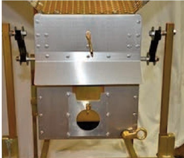
3. Flow control gate is located under classifier screen adjust with out of balance eye-bolt at the lower end of the classifier screen. This is used to control the feed into the recovery tray. We suggest that you run this at an 80% closed position. Material will continue to flow since the gate is made with fingers so the material flows consistently.
