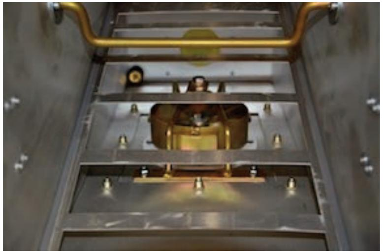
Next Slide the Riffle cartridge under the lip located just under the scrubbing pins.
